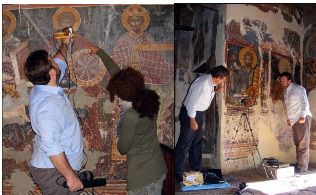
Fig. 5. In-situ examinations with the EDXRF instruments
